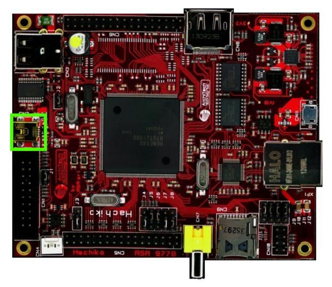
which you can connect, by means of a mini-USB cable, to your personal computer.
